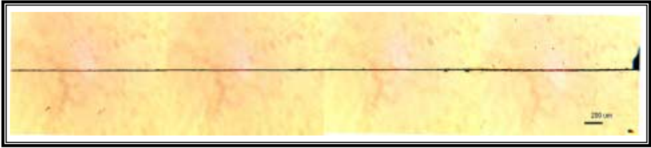
Figure 3: OLM image montage of the silicon surface after edge polishing. The combined abrasive suspension / diamond film process exhibits a superior surface finish than those previously obtained in this report.
